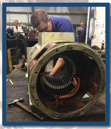
Fully Certified to service FLAMEPROOF Ex apparatus to AEMT standards inline with ATEX directive
