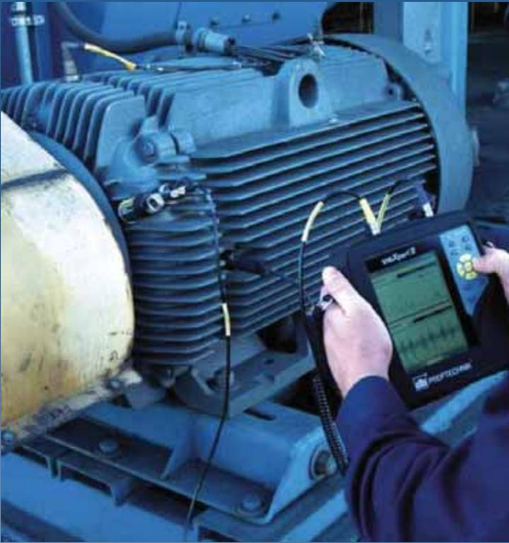
Through periodic monitoring of machines vibration, problems such as bearing wear can be detected early enough to permit planned repairs instead of unexpected break downs.
