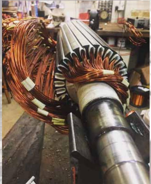
**D.C. electric motor repairs & armature rewinds**
